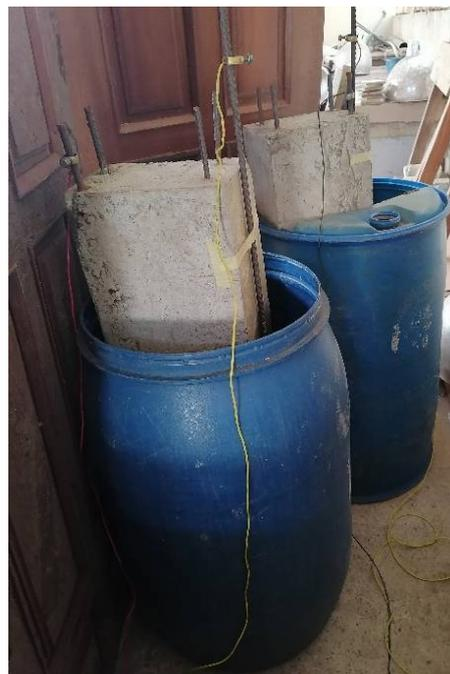
Figure 5. Simulated corrosion set-up in the laboratory.
