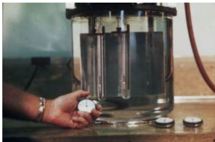
Figure 3.1.4 Viscosity test on Bitumen
