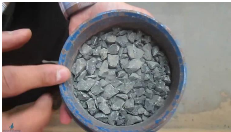
Figure 3.2.1 Impact test on aggregates
