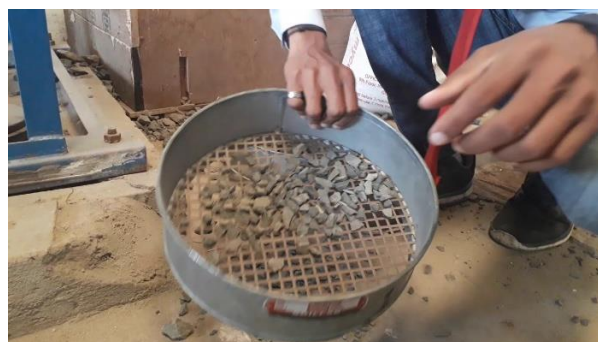
Figure 3.2.2 Abrasion test on aggregates
